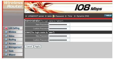
Administrator: Type the password the Administrator will use to log in to the system. The password must be typed again for confirmation. The authority if Administrator allow user configuration of the WLAN Router.
